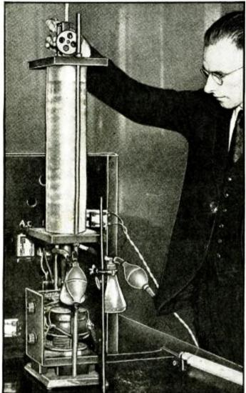
Fig. A. Sound-wave nodes and loops are visualized in ammonium chloride vapor.
